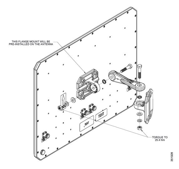
Figure 6 Assembling the Bracket Hardware
